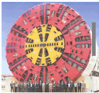
A Tunnel Boring Machine (TBM)
